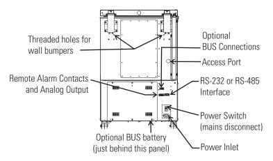
Figure 1-3. Rear View 3 cu ft Models
