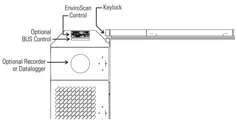
Figure 1-2. Front View Remaining Models
