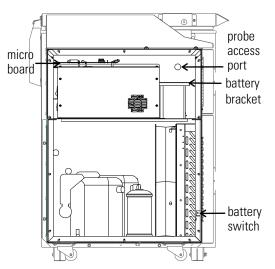
Figure 1-7. Freezer Left Side - Sidecar panel removed
