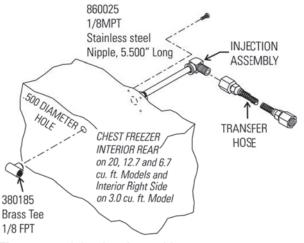
Figure 6-2. Injection Assembly
