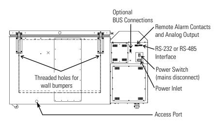
Figure 1-4. Rear View Remaining Models
