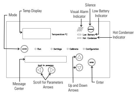
Figure 1-9. Control Panel Keys, Display and Indicators
